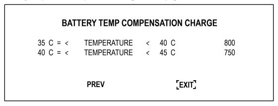
To edit the Battery Temperature Compensation, select the second line from the top in **Figure 93** and press the SELECT button. The following screen will come up.
